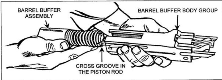
Figure 071-022-0001-18. Removal of the barrel buffer assembly
