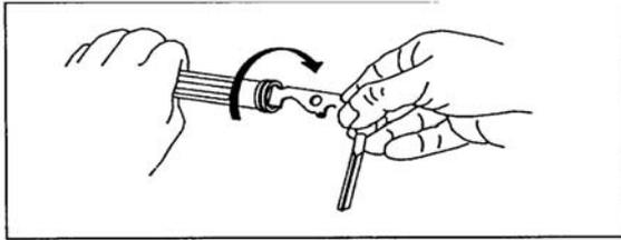
Figure 071-312-4025-18. Cleaning of the gas cylinder's internal grooves
