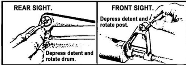
Figure 071-311-2004-2. Rear sight detent and front sight detent
