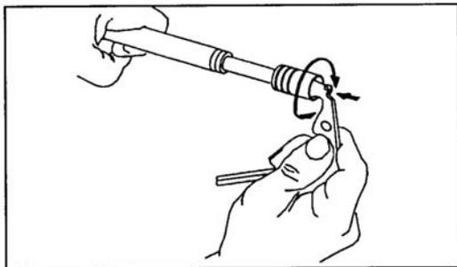
**Figure 071-312-4025-21. Cleaning of the hole in the piston**
