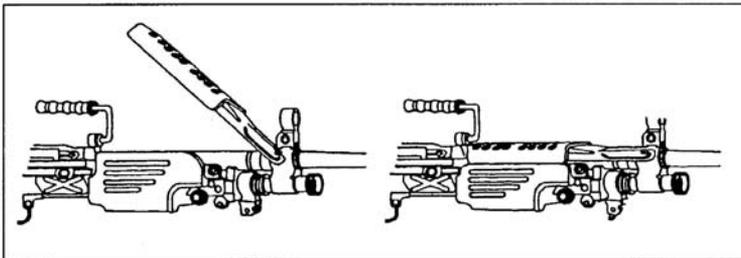
Figure 071-312-4025-35. Replacement of the heat shield assembly
