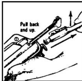
Figure 071-311-2025-10. Removing the bolt carrier and bolt
