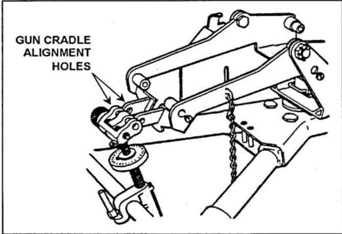
Figure 071-030-0011-5. Alignment of gun cradle to T&E
