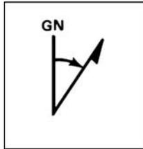
**Figure 071-329-1009-3. Converting azimuths with easterly G-M angle**
