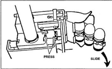
**Figure 071-030-0006-2. Removal of linked rounds from the feeder**
