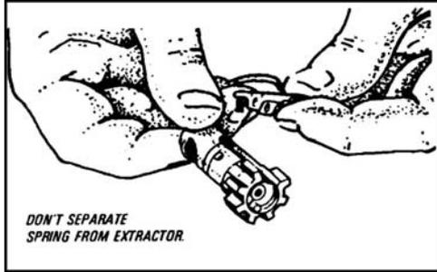
Figure 071-311-2025-18. Removing the extractor and spring
