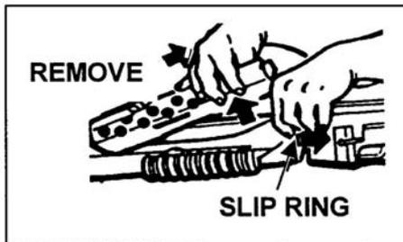
Figure 071-311-2125-3. Removing handguards
