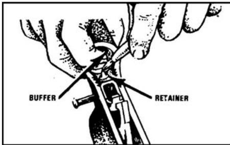
Figure 071-311-2025-19. Separating the buffer and spring
