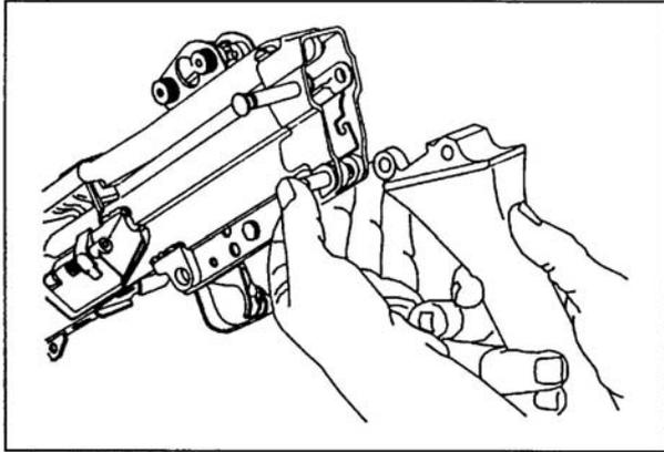
**Figure 071-312-4025-28. Replacement of the buttstock and shoulder assembly**
