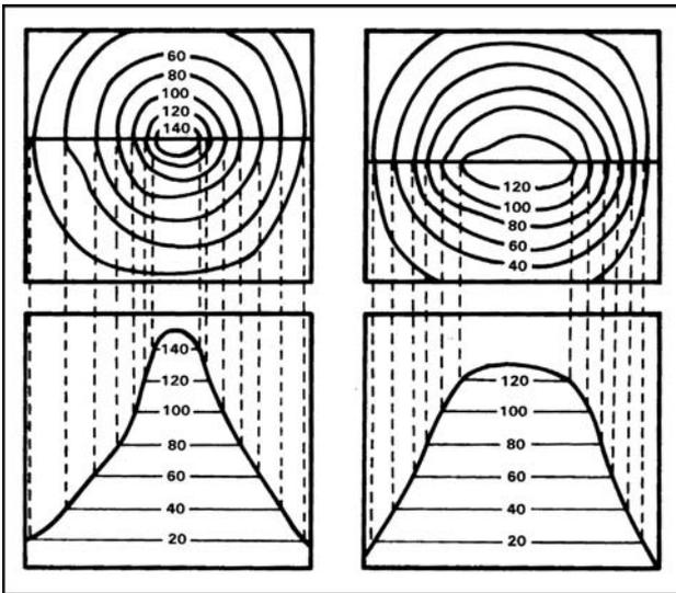
Figure 071-329-1004-4. Elevation
