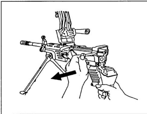
Figure 071-312-4025-1. Rear opening of the receiver
