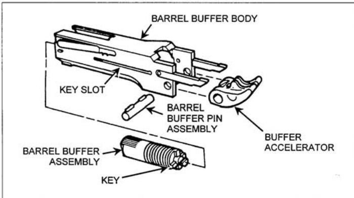
**Figure 071-022-0001-27. Assembly of the barrel buffer assembly**
