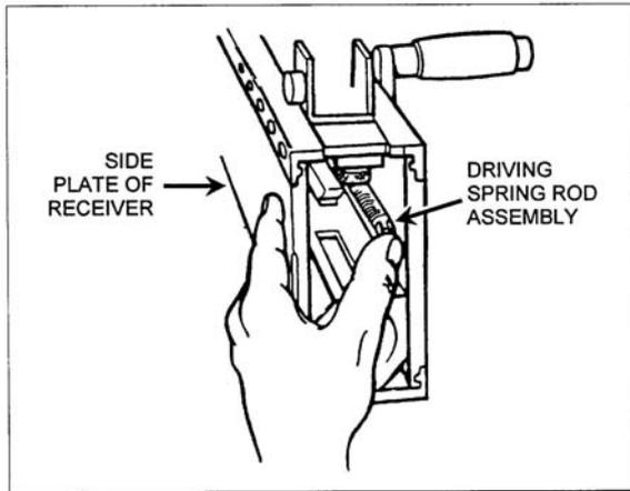
**Figure 071-022-0001-41. Installation of the driving spring rod assembly**
