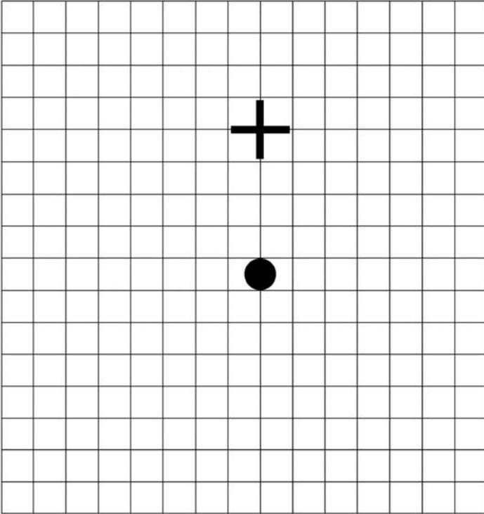
At a range of 10 meters aim at the cross and adjust the CCO so that the bore light strikes the dot.
