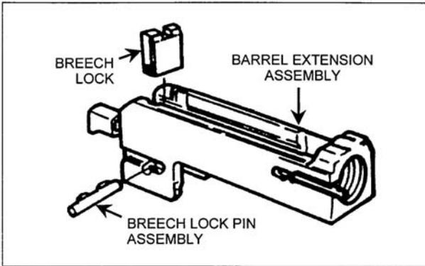
**Figure 071-022-0001-26. Assembly of the barrel extension assembly**
