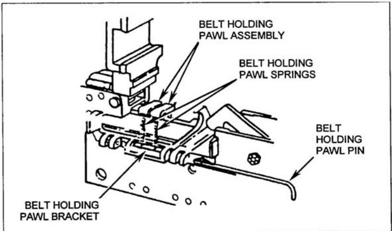
Figure 071-022-0001-25. Installation of the belt-holding pawl assembly
