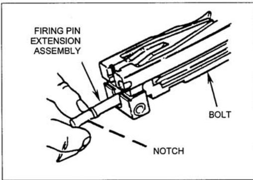
**Figure 071-022-0001-31. Installation of the firing pin extension assembly**
