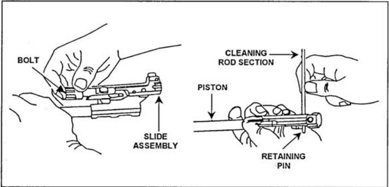
Figure 071-312-4025-5. Removal of the bolt and piston
