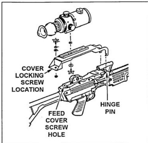
**Figure 071-010-0002-1. Installation of mounting bracket assembly**
