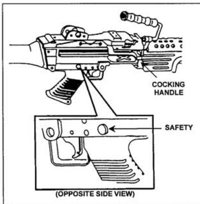
Figure 071-312-4027-1. M249 locking handle and safety
