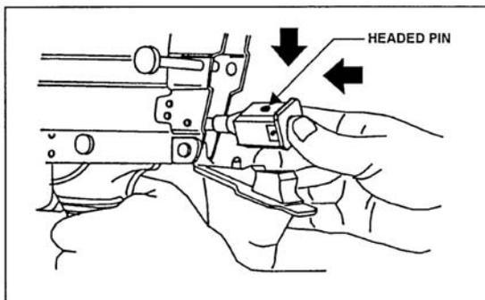
Figure 071-312-4025-33. Replacement of the return rod and transfer mechanism assembly
