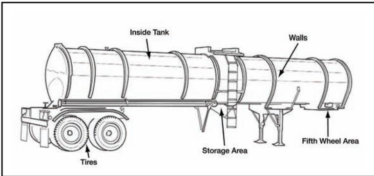
Figure 191-376-5141-6. Liquid tanker
