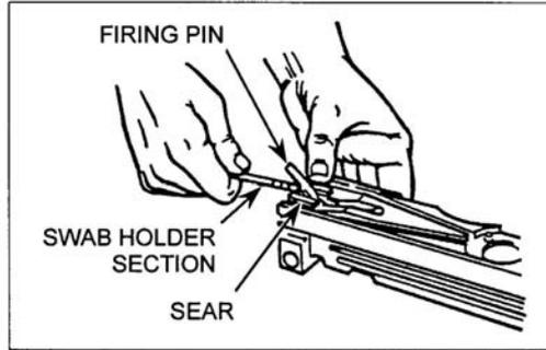
Figure 071-022-0001-36. Testing of the firing pin release
