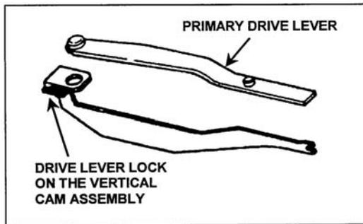
Figure 071-030-0001-4. Primary drive lever and vertical cam assembly
