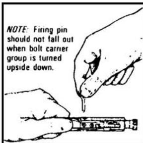
Figure 071-311-2025-30. Placing the firing pin retaining pin
