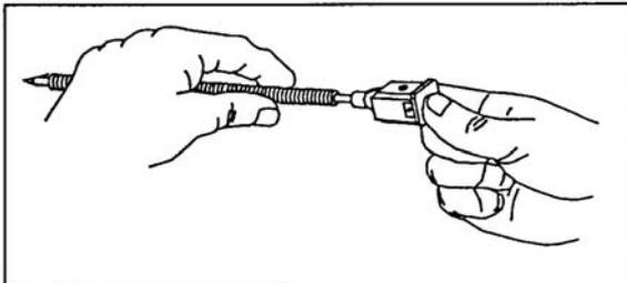
Figure 071-312-4025-32. Replacement of the spring
