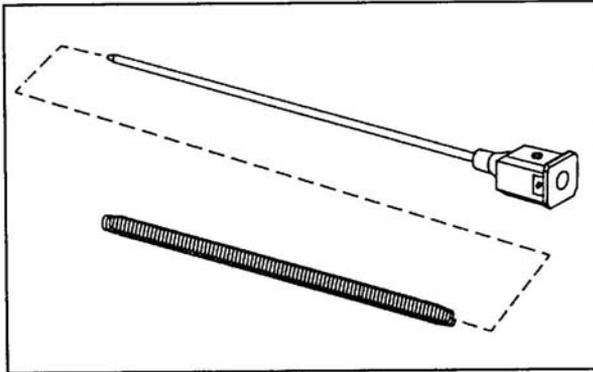
Figure 071-312-4025-3. Removal of the spring
