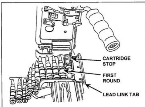
Figure 071-312-4027-4. Link belt in the feed tray
