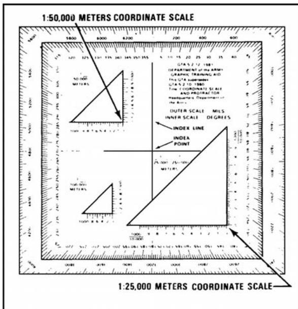
Figure 071-329-1002-4. Plotting scale
