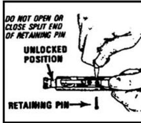
Figure 071-311-2025-12. Removing the firing pin retaining pin
