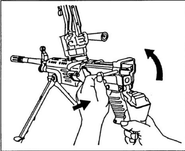
Figure 071-312-4025-34. Cleaning of the rear of the receiver
