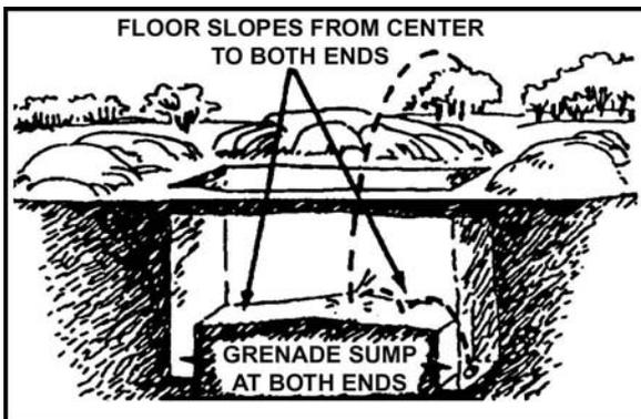
Figure 071-326-5703-6. Two trench-shaped grenade sumps
