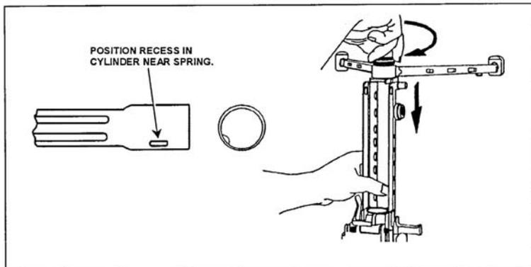
**Figure 071-312-4025-22. Replacement of the bipod and gas cylinder**
