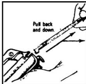
Figure 071-311-2025-11. Removing the charging handle
