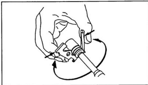
Figure 071-312-4025-20. Cleaning of the grooves of the piston
