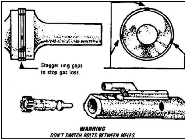
Figure 071-311-2025-27. Placing the bolt in the carrier
