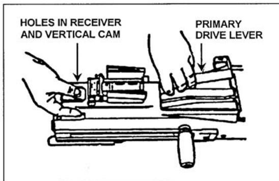
Figure 071-030-0001-23. Engagement the primary drive lever
