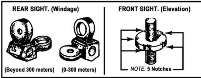
Figure 071-311-2004-1. Long-range aperture "L" on the rear sight
