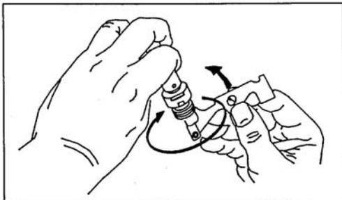
Figure 071-312-4025-17. Cleaning of the grooves of the regulator body
