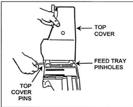
Figure 071-030-0001-20. Attachment of the top cover assembly
