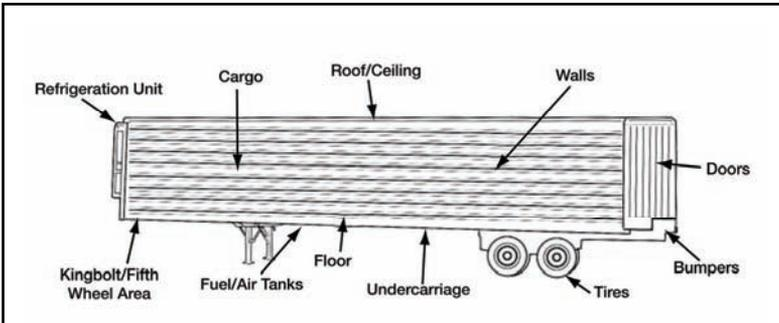
Figure 191-376-5141-10. Refrigeration trailer
