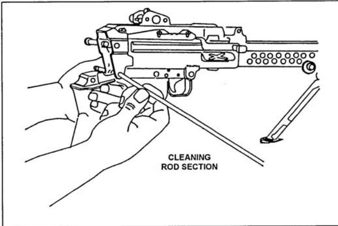
Figure 071-312-4025-11. Removal of the buttstock and buffer assembly
