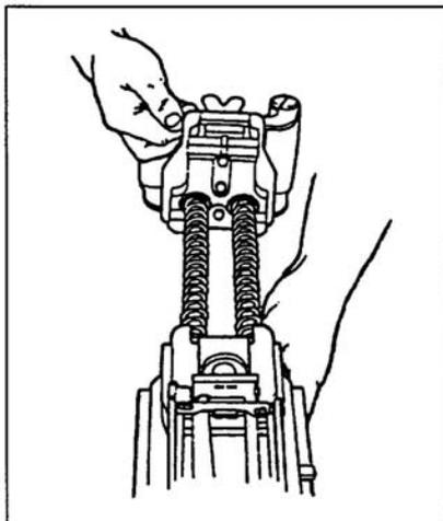
Figure 071-030-0001-3. Removal of bolt and backplate assembly
