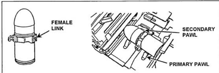
Figure 071-030-0005-1. Insertion of first round through feed throat
