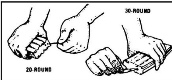
Figure 071-311-2025-40. Releasing the base catch of the magazine
