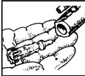
Figure 071-311-2025-16. Removing the bolt
