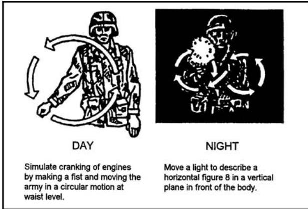
Figure 071-326-0608-21. Start engine, or Prepare to move
