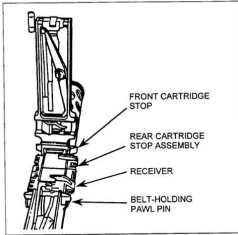
Figure 071-022-0001-20. Removal of the cartridge stop assemblies
