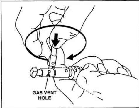
Figure 071-312-4025-15. Cleaning of the gas vent hole
