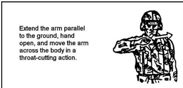
Figure 071-326-0608-31. Stop engines
