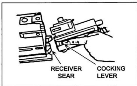
Figure 071-030-0001-24. Insertion of the bolt and backplate assembly
