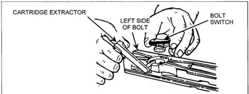
Figure 071-022-0001-9. Removal of the cartridge extractor and bolt
