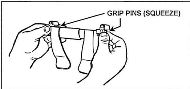
Figure 071-030-0011-10. Gripping of pins on feed throat assembly
