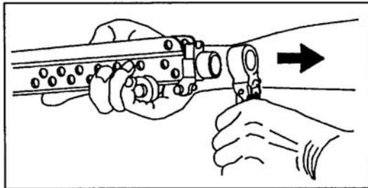
Figure 071-312-4025-14. Removal of the bipod
