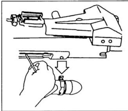
**Figure 071-030-0006-1. Removal of round or spent case**
