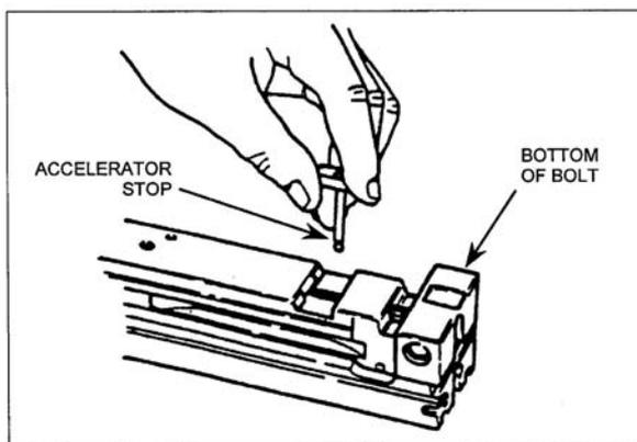
**Figure 071-022-0001-33. Attachment of the accelerator stop**
