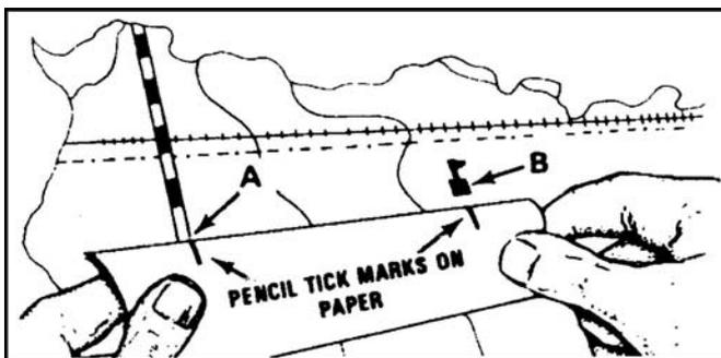
Figure 071-329-1008-2. Measuring distance
