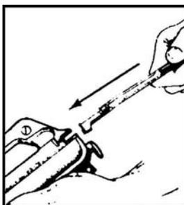
Figure 071-311-2025-32. Placing the charging handle in the receiver
