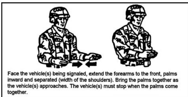
Figure 071-326-0608-30. Close distance between vehicles and stop
