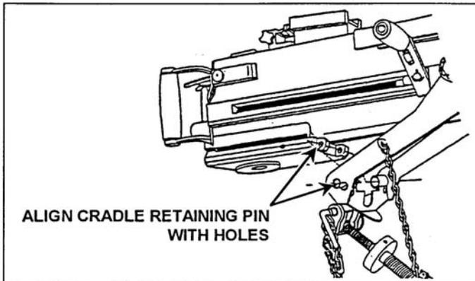
Figure 071-030-0011-8. Alignment of sear assembly, pin holes
