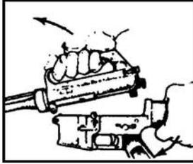
Figure 071-311-2025-8. Separating the upper and lower receivers
