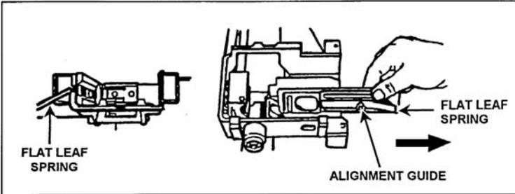
**Figure 071-030-0001-10. Removal of the alignment guide assembly**
