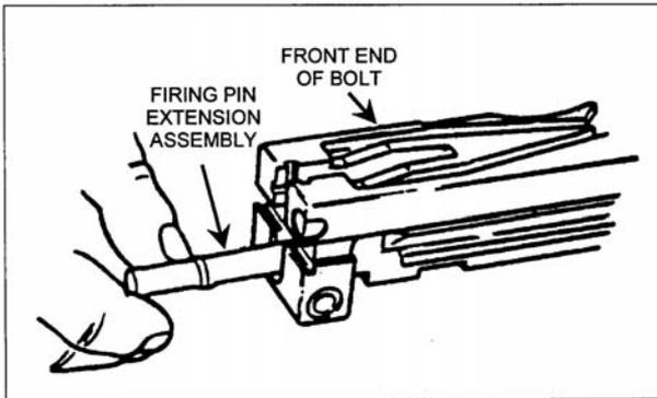
Figure 071-022-0001-15. Removal of the firing pin extension assembly
