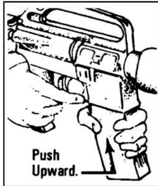
Figure 071-311-2027-3. Magazine inserted
