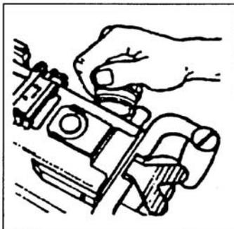
Figure 071-030-0001-2. Removal of backplate pin
