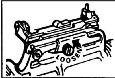
Figure 071-311-2125-2. Removing quadrant sight
