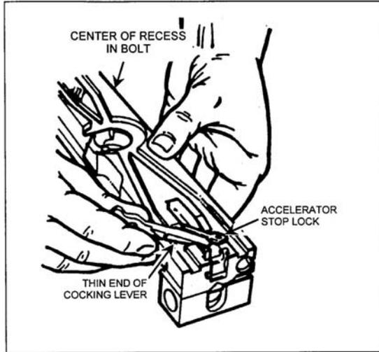
Figure 071-022-0001-12. Removal of the accelerator stop lock
