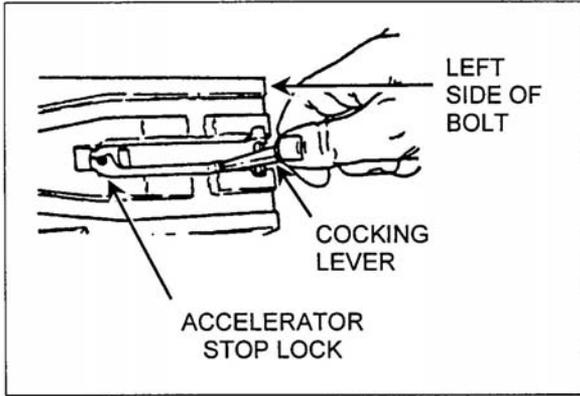
Figure 071-022-0001-34. Attachment of the accelerator stop lock
