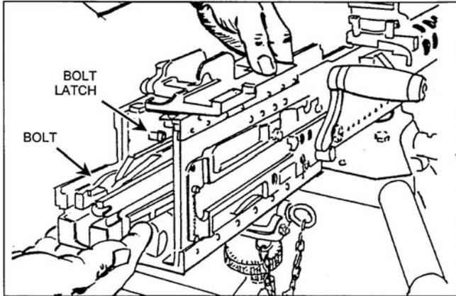
Figure 071-022-0001-8. Removal of the bolt from the receiver
