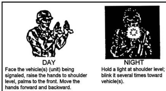
Figure 071-326-0608-29. Move in reverse (for stationary vehicles)
