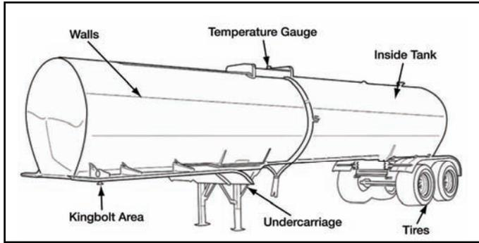
**Figure 191-376-5141-3. Hot-liquid asphalt tanker**
