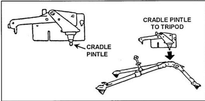
Figure 071-030-0011-3. Insertion of pintle into pintle bushing
