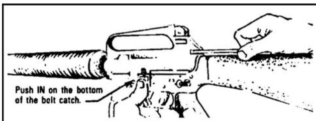
Figure 071-311-2027-006. Bolt locked to the rear
