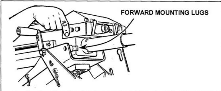
Figure 071-030-0011-7. Sliding of gun onto mounting lugs
