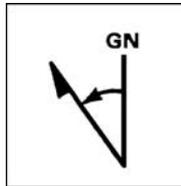
**Figure 071-329-1009-4. Converting azimuths with westerly G-M angle**
