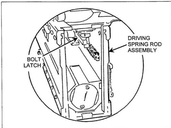
Figure 071-022-0001-5. Removal of the driving spring rod assembly
