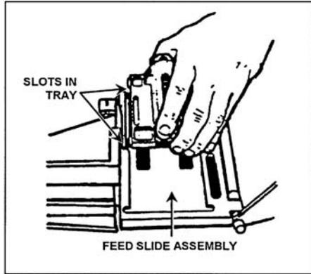
**Figure 071-030-0001-8. Removal of the feed slide assembly**
