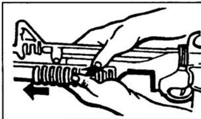
Figure 071-311-2125-4. Unlocking and opening the M203 barrel
