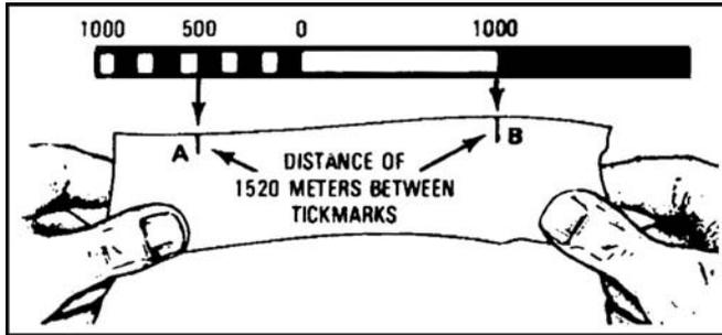
Figure 071-329-1008-3. Determining distance
